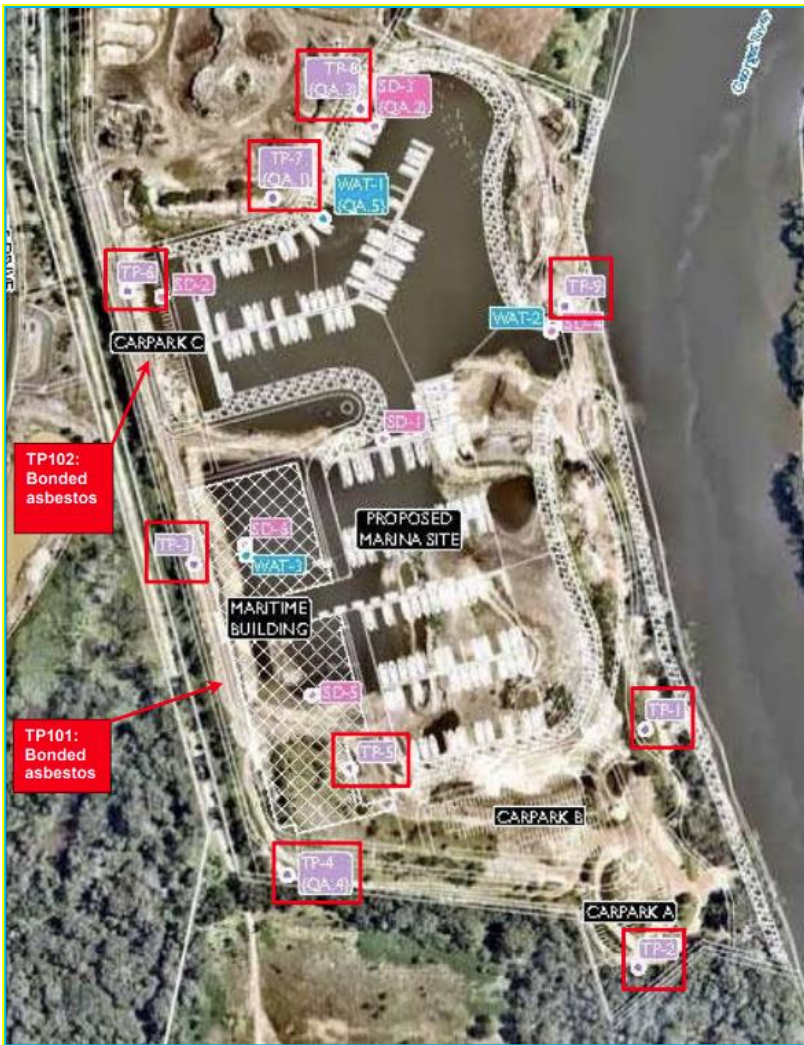
Figure 3.1 Locations of bonded asbestos fragments reported at the Marina site
